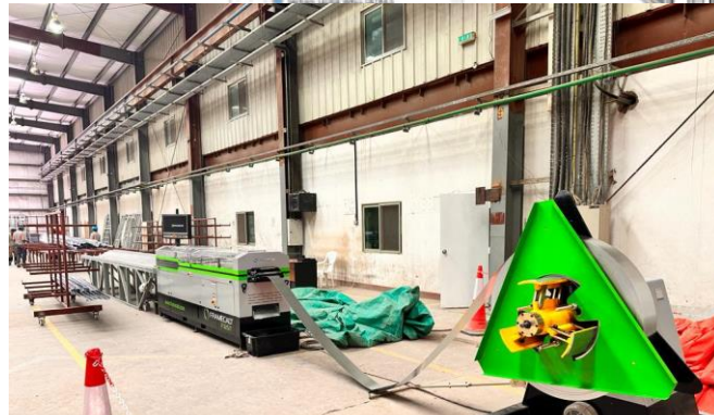
Framework production at our Modular Factory using roll forming machine
